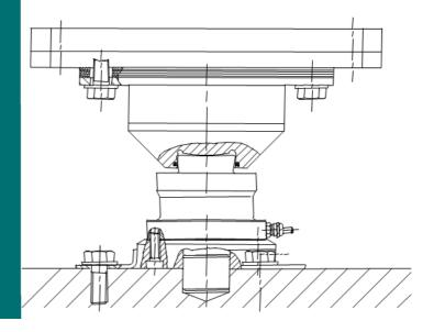
load distribution. The predefined packs extend the load cells' application temperature range to 150 °C.
