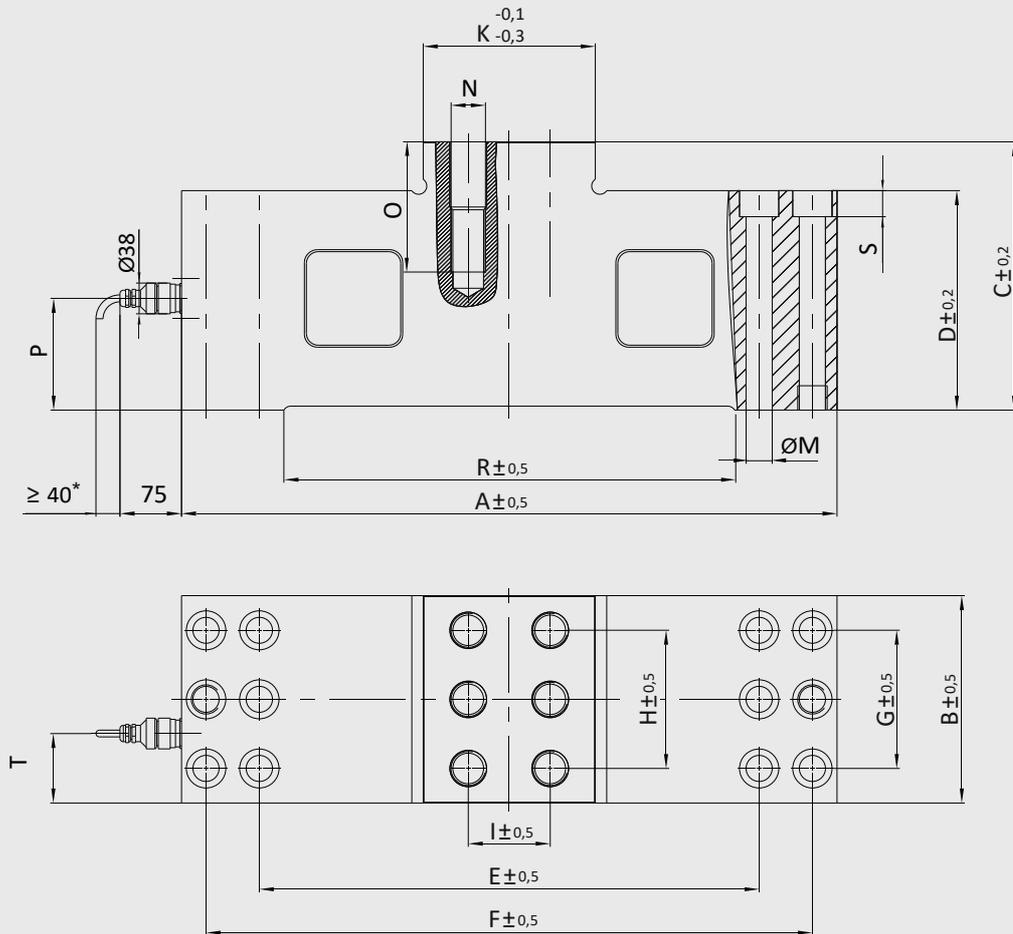
\* Another 15 mm are needed for isolating the plug connection.
